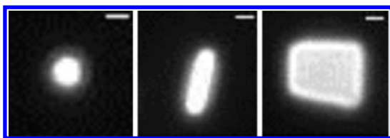
Figure 13. Single particle photoluminescence images obtained from movies of 25 s duration of \text{CH}_3\text{NH}_3\text{PbI}_3 nanocrystals with dot-, wire-, and plate-like morphologies (please see Supporting Information Movies S1, S2, and S3, respectively) ( \lambda_{\text{exc}} = 540 \text{ nm} , \lambda_{\text{PL}} = 700 \text{ nm} , scale bar = 1 \mu\text{m} ).
