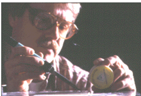
Ames Lab's new lead-free solder is an environmentally friendly replacement for the tin-lead solders that often end up contaminating landfills.
